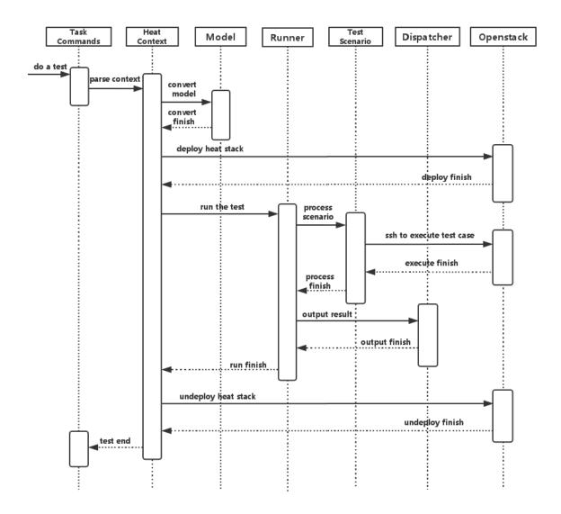
A user wants to do a test with yardstick. He can use the CLI to input the command to start a task. "TaskCommands" will receive the command and ask "HeatContext" to parse the context. "HeatContext" will then ask "Model" to convert the model. After the model is generated, "HeatContext" will inform "Openstack" to deploy the heat stack by heat template. After "Openstack" deploys the stack, "HeatContext" will inform "Runner" to run the specific test case.
