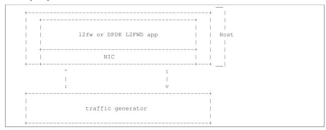
Benchmark VNF forwarding capability: This test is used to verify the VNF and measure the base performance
