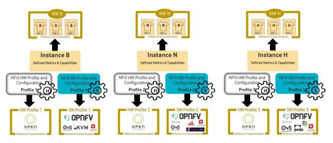
Figure 3.7: Reference NFVI Profiles Implementation
