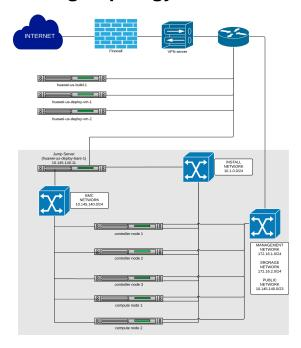
Figure 1: Huawei US lab OPNFV hosting environment overview
