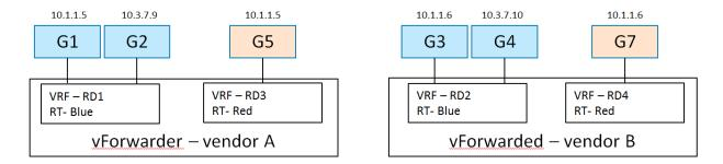
In L3VPN Blue, VMs G1 (10.1.1.5) and G2 (10.3.7.9) are spawned on host A, and attached to 2 subnets (10.1.1.0/24 and 10.3.7.0/24) and assigned IP addresses respectively. VMs G3 (10.1.1.6) and G4 (10.3.7.10) are spawned on host B, and attached to 2 subnets (10.1.1.0/24 and 10.3.7.0/24) and assigned IP addresses respectively.
