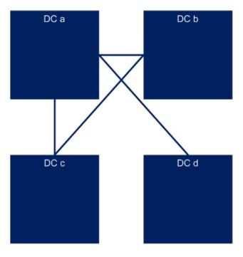
Each datacenter (DC) is a separate OpenStack cell, region or instance. Let's assume that a new VNF is started in DC b with a Redundant VNF in DC d. In this case a direct underlay network connection is needed between DC b and DC d. The configuration of this connection should be programmable in both DC b and DC d. The result of the deployment is shown in the following figure (Fig. 2.5):
