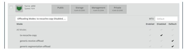
2. Set up targets for "Verify Networks" with non-default "Offloading Modes"
