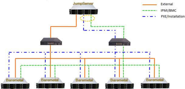
If jumpserver doesn't have enough ethernet ports, two ports is also acceptable(IPMI/BMC and PXE/Installation run through one ethernet port).
