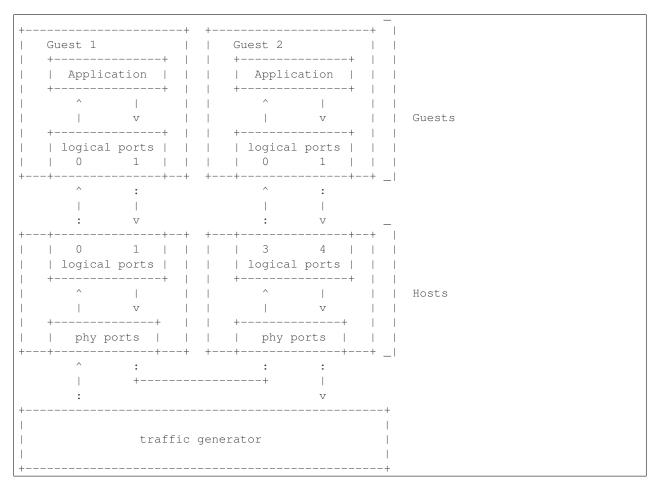
**Note:** For tests where the traffic generator and/or measurement receiver are implemented on VM and connected to the virtual switch through vNIC, the issues of shared resources and interactions between the measurement devices and the device under test must be considered.
