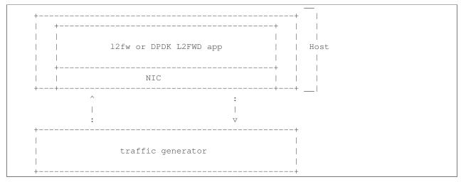
Benchmark VNF forwarding capability: This test is used to verify the VNF and measure the base performance (maximum forwarding rate in fps and latency) that can be achieved by the VNF without a vSwitch. The performance metrics collected by this test will serve as a key comparison point for NIC passthrough technologies and vSwitches. VNF in this context refers to the hypervisor and the VM. The following diagram outlines the set-up for benchmarking VNF forwarding capability:
