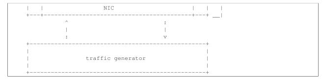
• Benchmark VNF forwarding capability: This test is used to verify the VNF and measure the base performance (maximum forwarding rate in fps and latency) that can be achieved by the VNF without a vSwitch. The performance metrics collected by this test will serve as a key comparison point for NIC passthrough technologies and vSwitches. VNF in this context refers to the hypervisor and the VM. The following diagram outlines the set-up for benchmarking VNF forwarding capability:
