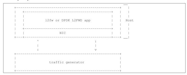
Benchmark VNF forwarding capability: This test is used to verify the VNF and measure the base performance (maximum forwarding rate in fps and latency) that can be achieved by the VNF without a vSwitch. The performance metrics collected by this test will serve as a key comparison point for NIC passthrough technologies and vSwitches. VNF in this context refers to the hypervisor and the VM. The following diagram outlines the set-up for benchmarking VNF forwarding capability:
