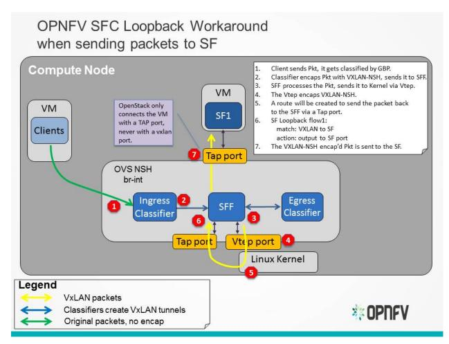
The following diagram illustrates how packets will sent from an SF to an SFF, once the SF has processed a packet:
