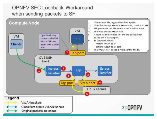
The following diagram illustrates how packets will sent from an SF to an SFF, once the SF has processed a packet:
